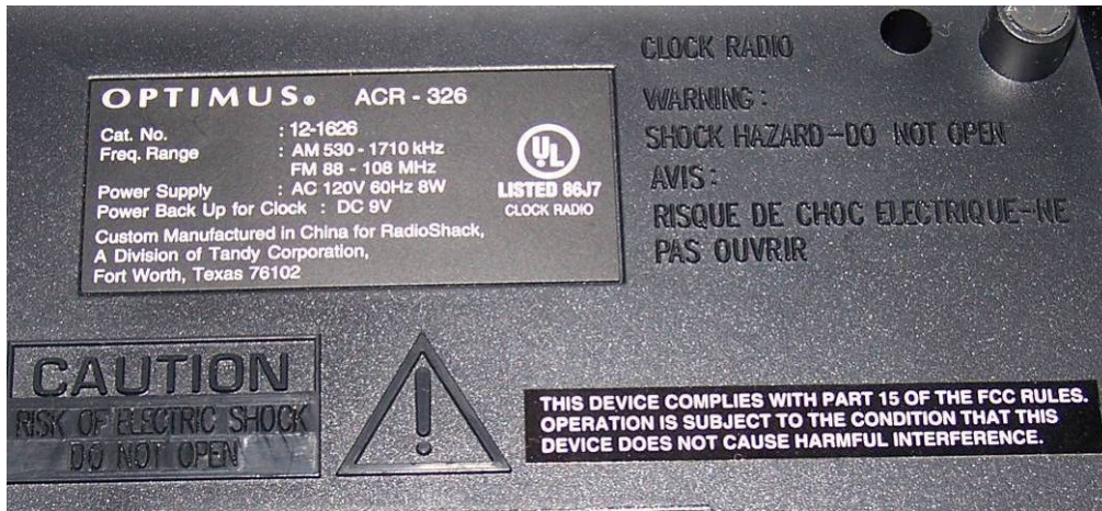
Figure 38 - Part 15 Label from a Clock Radio. Photo by N5IUT
