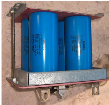
Figure 59 - Power Supply capacitors. Photo by N5IUT
